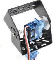
Pan/Tilt Servos (two needed per bracket) 100 Servo-Generic (Sub-Micro Size)
