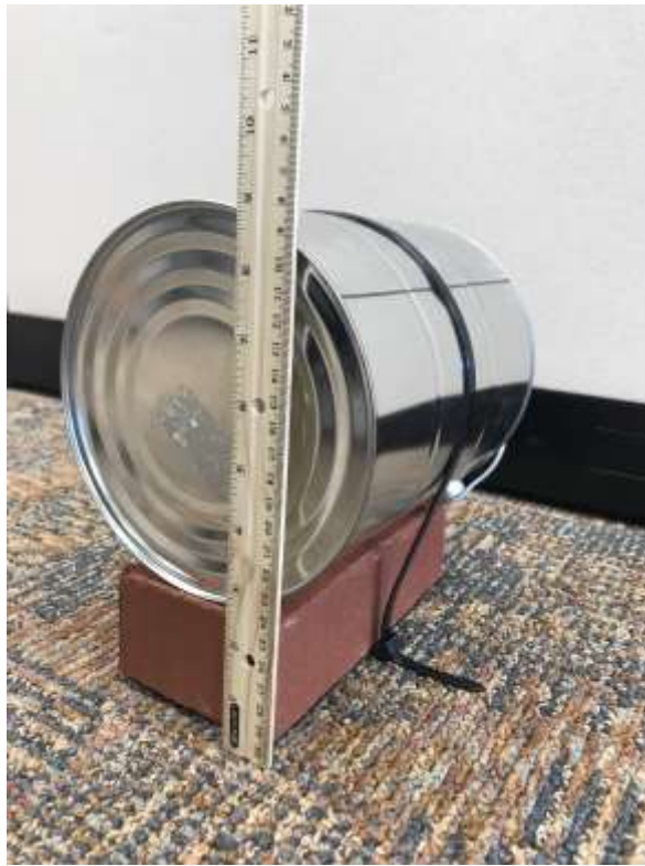
Drum: Strike Height 2" above the ground (gallon paint can)
