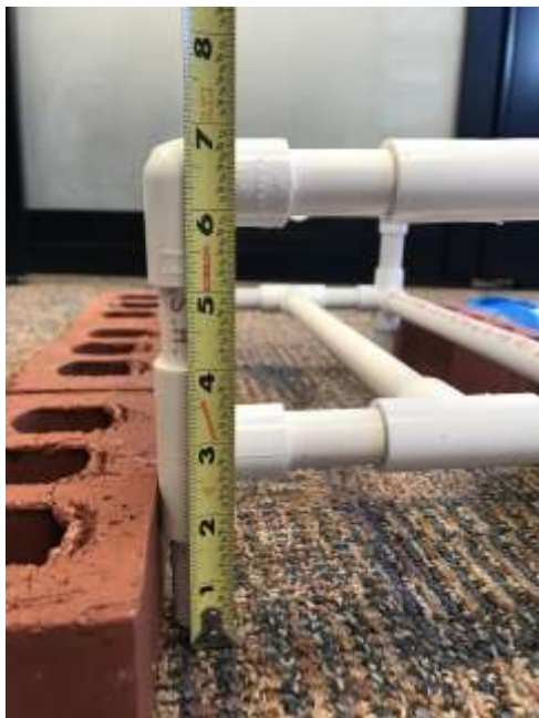
Coin Activator: \frac{1}{2} " pvc pipe, 16" X 8" x 7"
