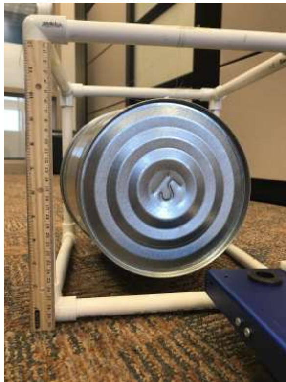
Gong: Strike Height- 2" above the ground (lowes 12 qt. General bucket)
