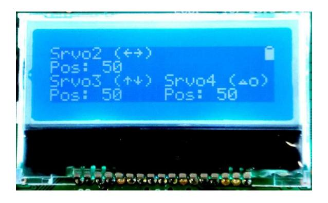
The screen is split into three areas for the three servos. The upper left area shows servo 0 details, including a cue to use the remote control cross left and right buttons, and the current position of the servo (from 0 to 100).
