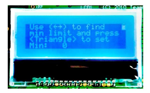
We suggest first setting the stepping speed to low so you have more control over the servo's motion. Then move the servo one button press at a time until it either reaches the location needed for the project, or until the servo will no longer turn. If you reach the lower limit of the servo and still need to turn the servo further, step the servo back to a value where it moves. Then remove and adjust the hardware attached to the servo and re-install it at the minimum position.
