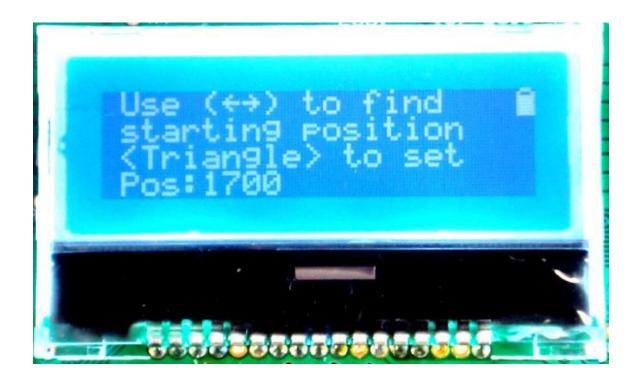
When the servo is where you want it, press the triangle button to save all settings and return to the servo information screen.
