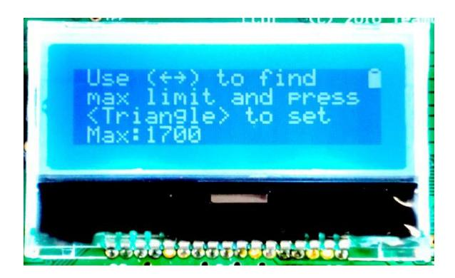
Once the servo and the hardware are where you want them, and the servo is NOT turned beyond it's limit, press the triangle button on the remote.
